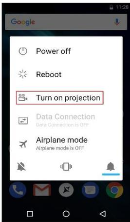
To close the projection, press for 2 seconds the Power button and choose *Turn off projection*:
